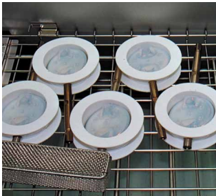
Cleansing the parts with ultrapure water
