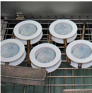
Cleansing the parts with ultrapur water
