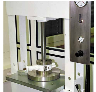
Thightness test with ultrapure air
