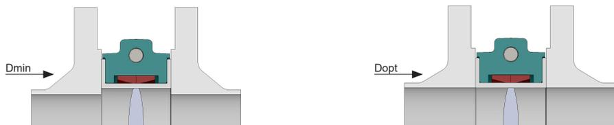
Dmin Minimum diameter of the flange enabling to move the disc (in case of a perfectly centered valve)
